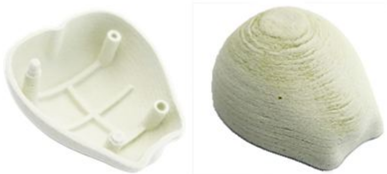
Figure 5.1. Experimentally printed part via ink jet
