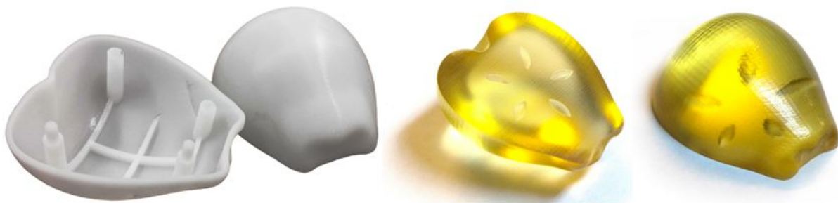
Figure 5.2. SLA (left) and PolyJet (right) printed parts
